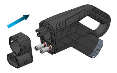
Setp 6: Tighten 5 Torx M4\*50 screws, the recommended tightening torque is 1Nm, and fix the gun head frame
